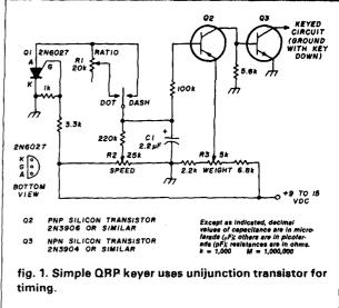
of Q2 is direct-coupled to Q3, the switching or keying transistor. R3, the "weight" potentiometer in the emitter of Q2, controls the switching threshold (the onoff periods) of Q2 and Q3.
